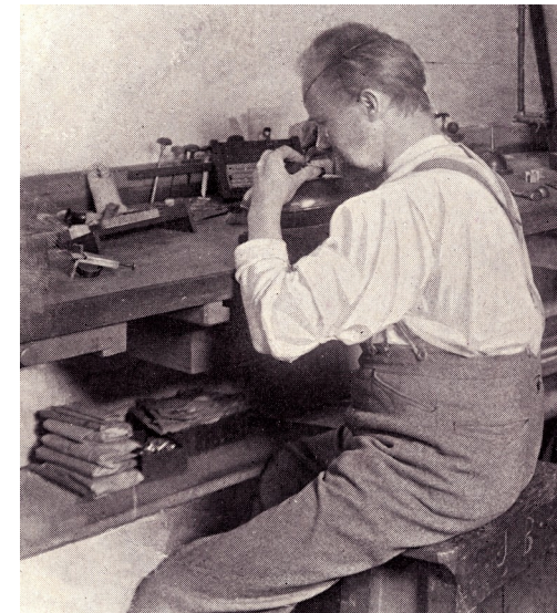
Hand matrix engraving at the Philadelphia foundry (C) of ATF (ex-MSJ). From One Hundred Years (1896).
