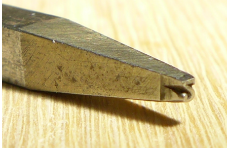
A punch, probably hand-cut. Thompson Type Machine Co.
