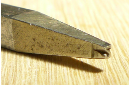
A punch, probably hand-cut. Thompson Type Machine Co.
