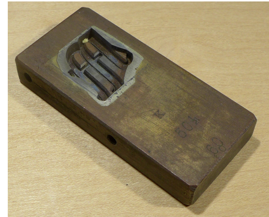
An Electroformed Matrix. ATF Series 476 Goudy Handtooled Italic. 60 point. For the Barth Type Caster.
