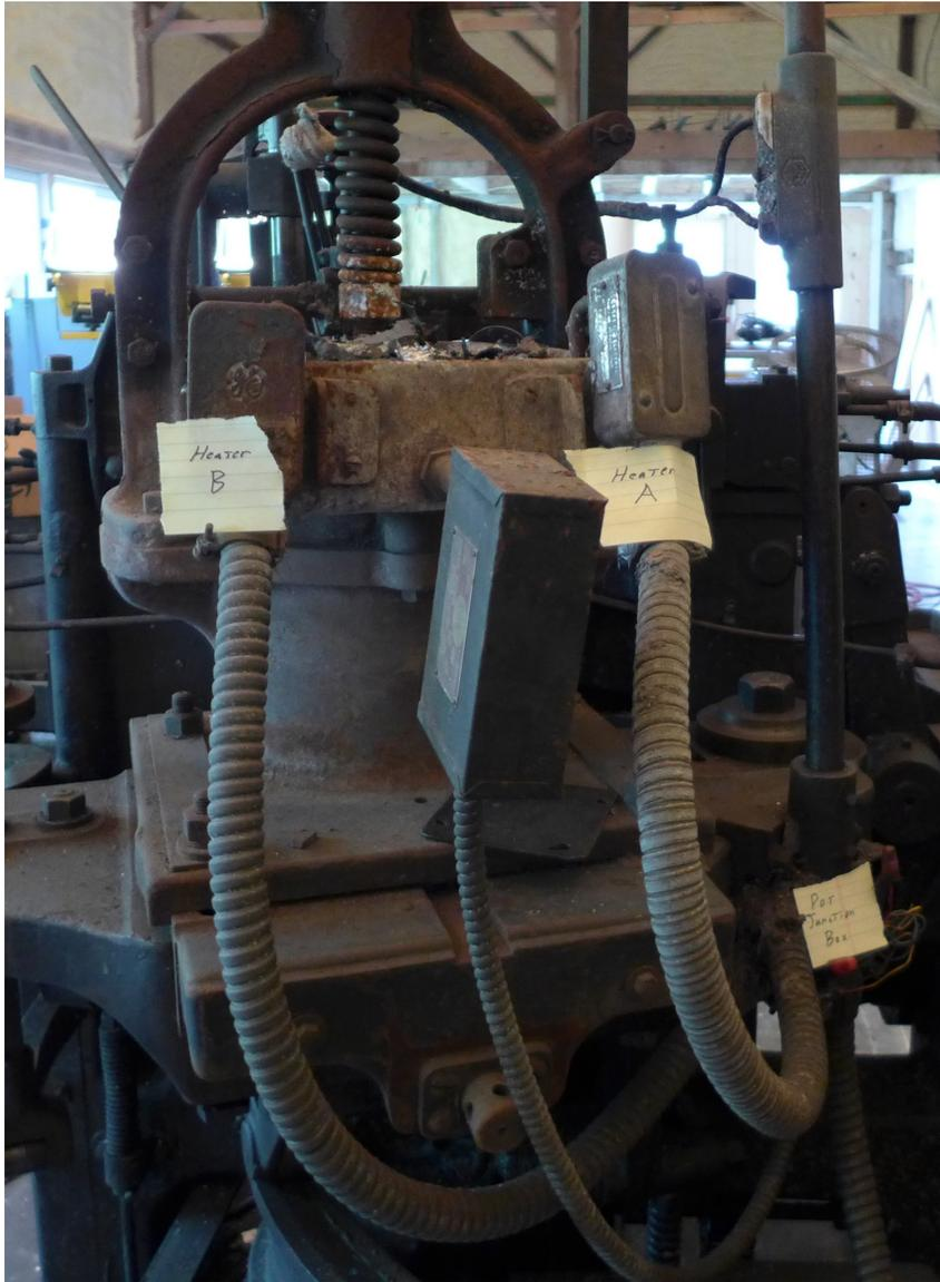
A view from behind the caster of Pot Heater 'A' (on the right in the photo, which is on the left / flywheel side of the machine as viewed from the front) and Pot Heater 'B' (at left in the photo).
