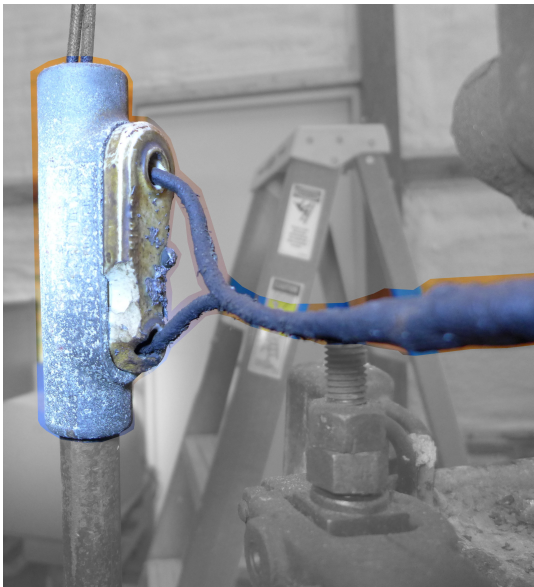
91bcd23 Throat Heater Assembly (right photo) and its wiring from the 91BCD14 Pot Heater Lamp Standard Tee Condulet (left photo) Shown from the front (nipple side) of the Pot, with the Pot swung back.
