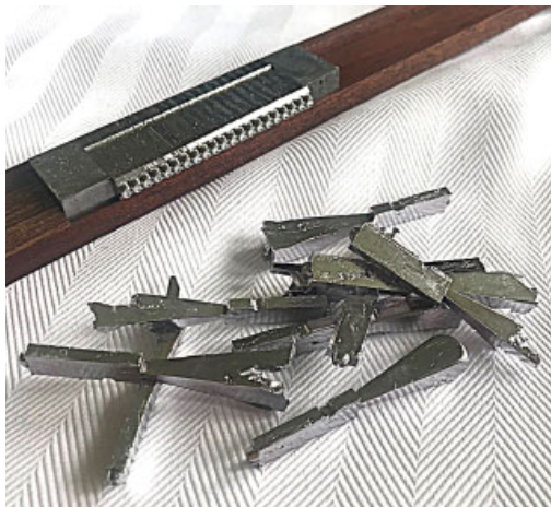
Below: Rough casts and finished type on a stick. At right an open mold with matrix in place.
