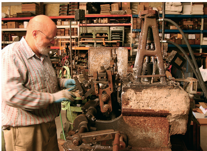
Greg at his pivotal caster with the mold half open for inspection.
