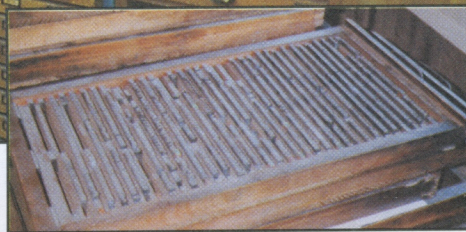
This drawer demonstrates how the Germans store larger sizes of type. Rather than in compartmentalized cases, the fonts are in drawers sometimes with dividers between lines, sometimes not. The photographer reports this drawer contains nothing but Egyptian Hieroglyphs. CHUCK KLENSCH
