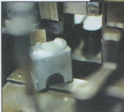
Casting machines of all types and sizes were on display at Leipzig. The very special mold in this machine enabled the casting of very large letters with a huge cut-away "groove." The open mold is in the background. RICH HOPKINS
