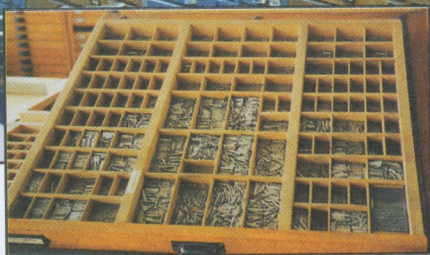
A standard typecase layout in Germany. Their cases have deeper compartments, and obviously more compartments in the rear in comparison with American typecases. LEONARD SPENCER
