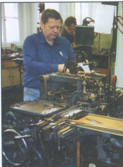
← No matter whether they're casting German or English, operation of the Monotype Composition Caster is the same.
