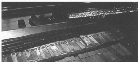
Foundry-style mats laid out to be cast. The Old Black mats are at top. Below is Stan Nelson's private face, Robin, which unfortunately did not get cast during the session.
