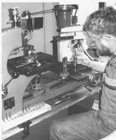
Hans Ulrich at the Engraving machine. It meets the highest requirement for precision, accommodating the tiniest cutters of a mere .0032 inch diameter.
