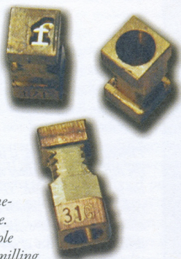
The English Composition matrix shown in four views: face, cone-hole end, flat side and side-hole side. The English cone-hole is more shallow than the American matrix. Drive of the matrix is .050", but the matrix was redesigned (as compared with original Lanston side-hole matrix) to allow for a steel supporting bar to go between matrices on the vertical axis.
