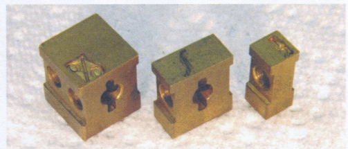
Double- and quad-sized matrices were made when letters exceeded the single matrix width or height—or both.
