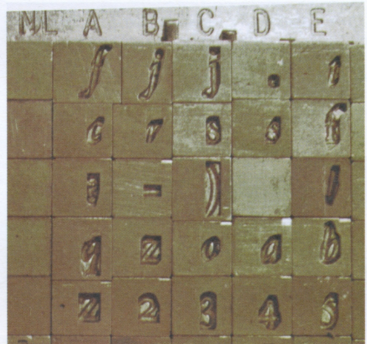
Assembling mats together in a matrix case where some letters exceed the 1/5 inch dimension becomes a true jigsaw puzzle. Notice the f exceeds both height and width. The italic j exceeds height but is made narrower to allow the wider f. The c and r are undersized. The parenthesis exceeds its size both at top and bottom.
