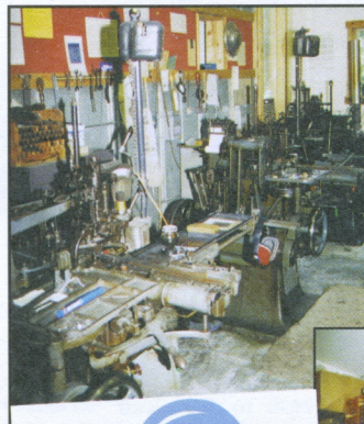
A partial view of the Monotype facilities housed in the barn at The Printing Farm. Here are three casters, along with a big inventory of composition and display matrices. Photos were taken by Paul Duensing during a visit in 1999.
