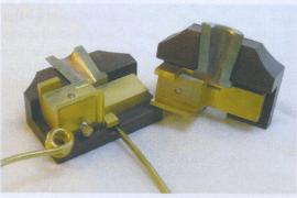
A precise replica of an early 16th century form of brass mold, based upon mold GI#48 in the Plantin-Moretus Museum, Antwerp. Stan made this particular mold for Wells College.
