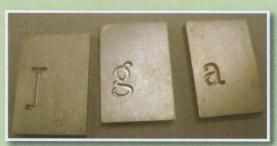
Here are three experimental brass mats Mel Arndt has made on his milling machine. With the naked eye the mats appeared very accurate and fit for the job, but a close-up of a casting (above) showed the cutting tool had problems which translated into rounded characters with a "fuzzy face." Photos by K. P. Martin
