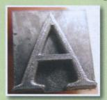
Very close examination of the cast type revealed problems which were not easily visible looking at the matrices. Mel explained the "chatter" visible on the face of the mats, along with rounded
