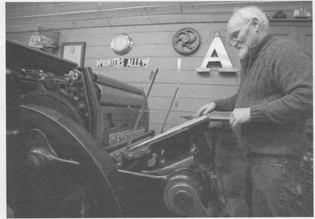
Found rusted shut in an open farm field, Jim knew the potential of the Colt's Armory Press and completely refurbished the machine, including making and machining several missing parts; Jim knew the press could deliver the strong, even impresssion needed for TOM SAWYER.
