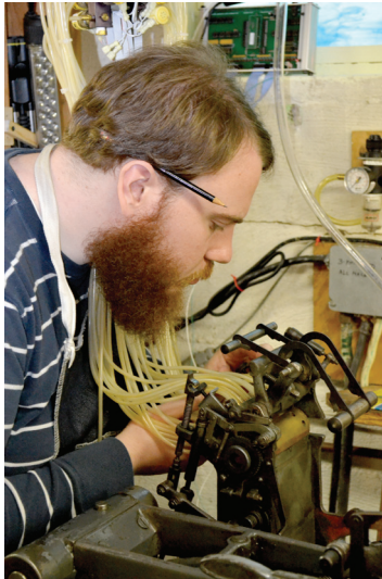
Joshua Steward adjusting the Computer Interface connection to the Paper Tower of the Casting Machine at Mono U 8.
