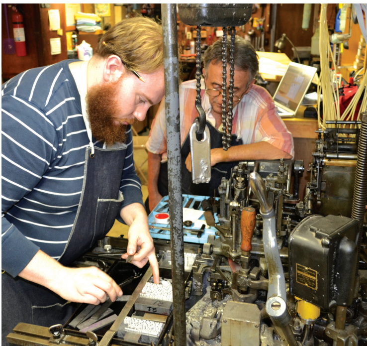
Joshua and Carl (he's behind all the pig-feeder chains) are retrieving a few paragraphs composed on this Composition Caster using the CompCAT Interface.
