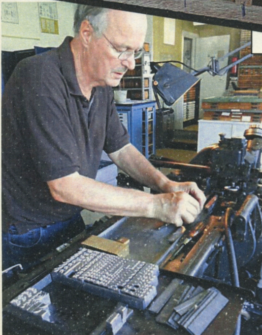
A huge brass sheet engraved with the various letter components is shown in the background. Overlaying is a box containing all matrices in finished form, cut from the master engraved sheet. To its right is a first proof of the typecast characters revealing various deficiencies in alignment (see text). To the left is Ronald Steur of Stichting Lettergieten 1983 at the Supercaster. Below are finished mats laid out.
