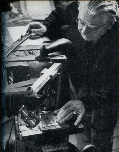
Exact reproduction of the master pattern, in type metal, one-third size, is cut on the router (lower table) while Mr. Goudy guides the "tracer" of a pantographic routing machine above.
