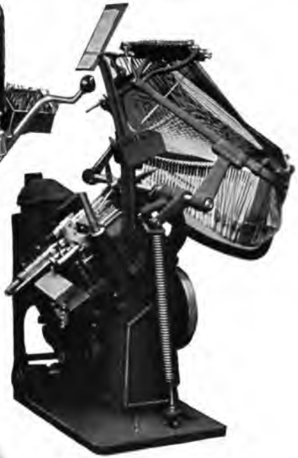
Fig. 106. Distributing position showing upper portion tilted back.
