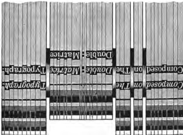
Fig. 107. Line of Two-letter Matrices Composed and Line-justified.
