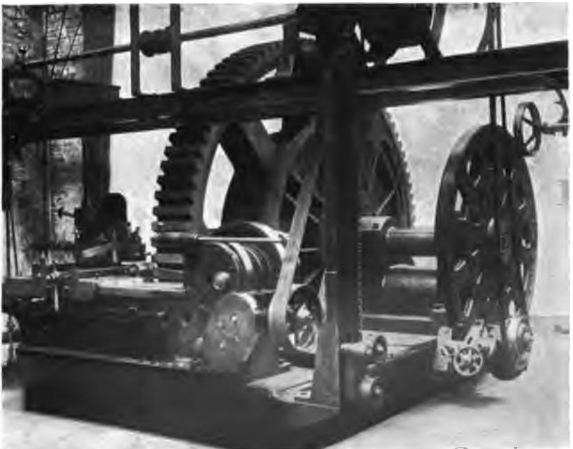
Fig. 21. Spur-Gear Planing Machine. (Gleason.)
