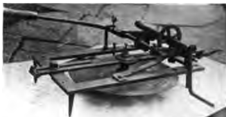
Fig. 9. Wheels with Machine cut Teeth. (Bodmer.) 1820-30.
