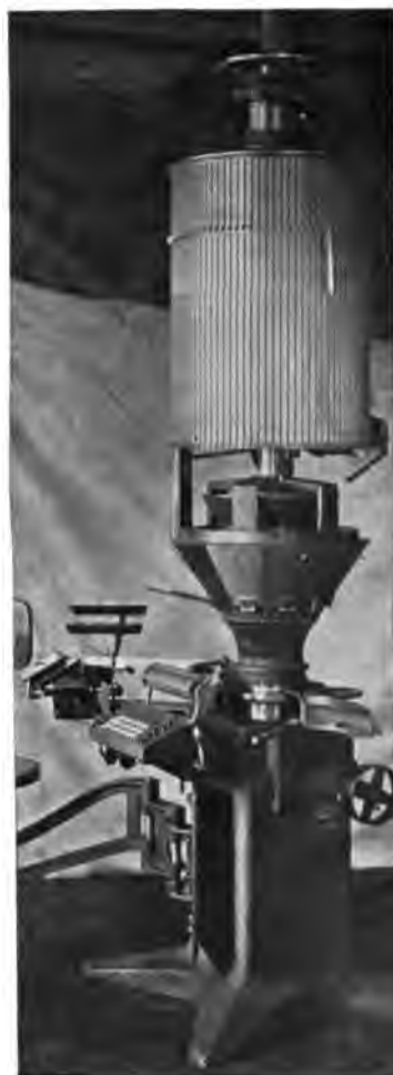
Fig. 127. Unitype Type distributing, Composing, and Line-justifying Machine (Thorne).
