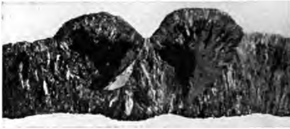
Fig. 11. Crystalline Structure of Deposited Copper.
