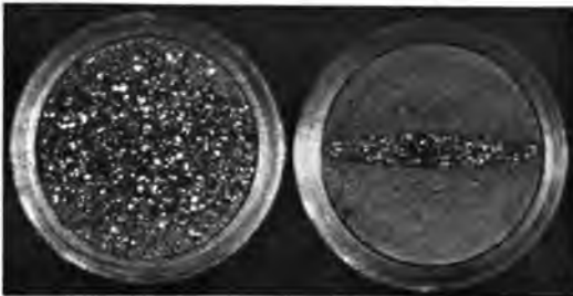
Fig. 37. Impact Tests on Specimens cut from a Fractured Crank-Shaft (Table 19). Untreated Specimen. Restored Specimen.
