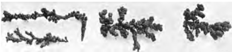
Fig. 12. Copper Trees, effect of Free Acid on Nodule Formation.
