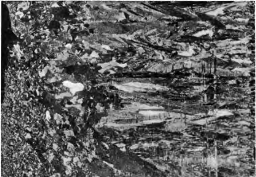
Fig. 12. Copper Trees, effect of Free Acid on Nodule Formation.
