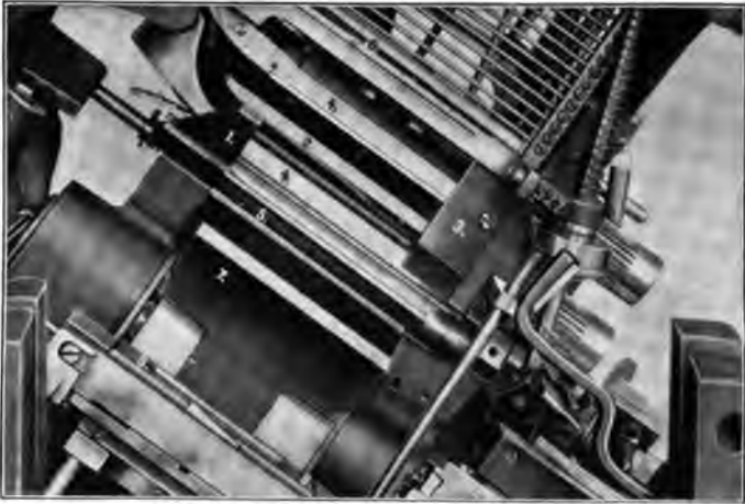
Fig. 119. Assembly Channel Empty.
