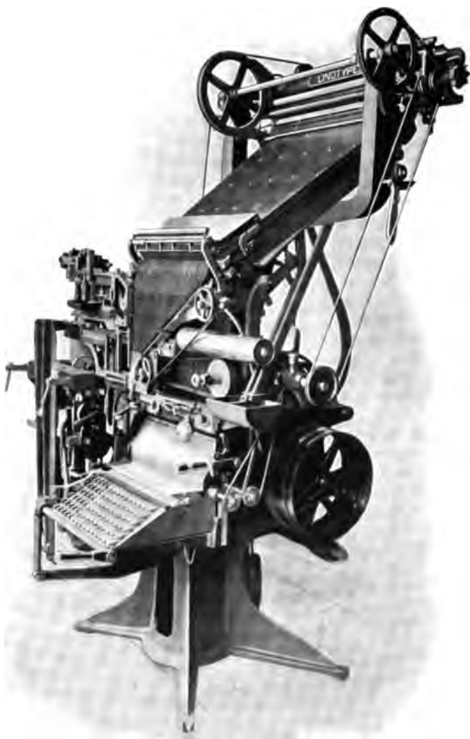
Fig. 102. Double Magazine Matrix Composing and Slug-casting Machine (Linotype).
