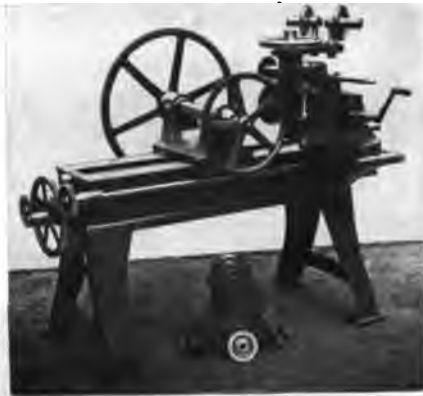
Fig. 15. Machine for Cutting Wheels. (Shepherd, Hill & Spink.) 1851.
