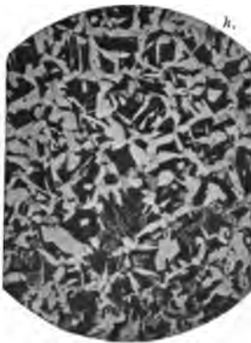
Fig. 36. Examples of the Relation between Size of Grain and Mechanical Properties. × 23 diams.
