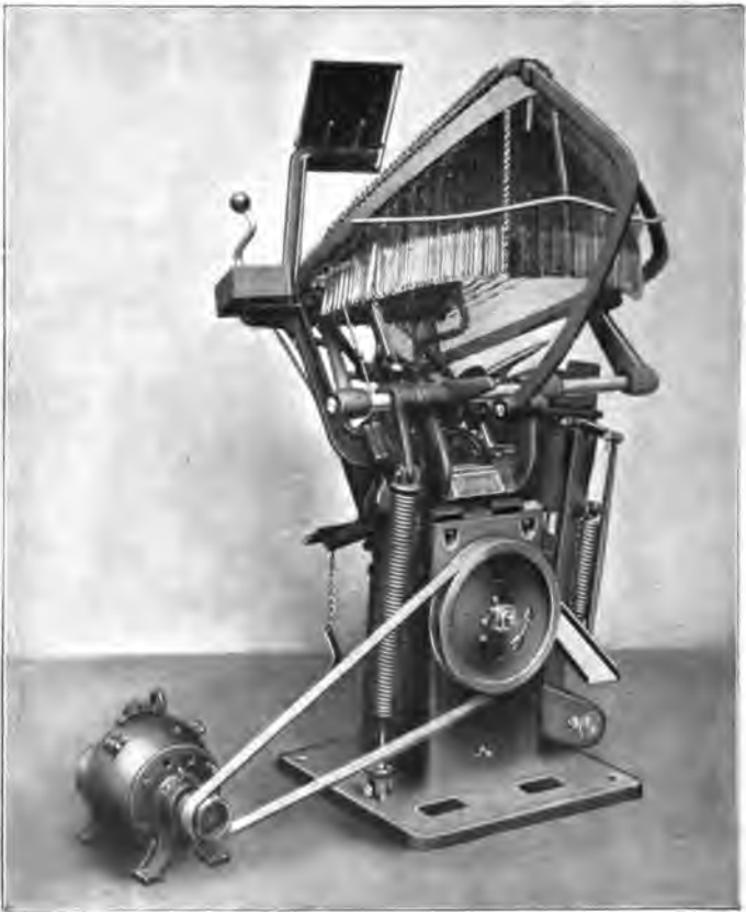
FIG. 434.— Typograph; normal composing position of upper part ; back view.
