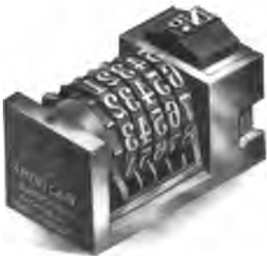
FIG. 319.—American numbering-machine and impression of figures.
