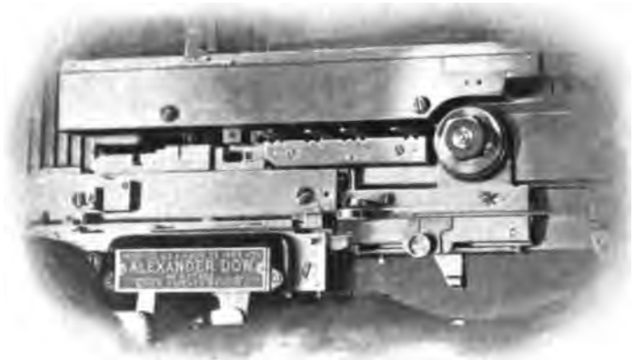
FIG. 346.—Dow composing machine; stick rotated through 90°; ejection of line.
