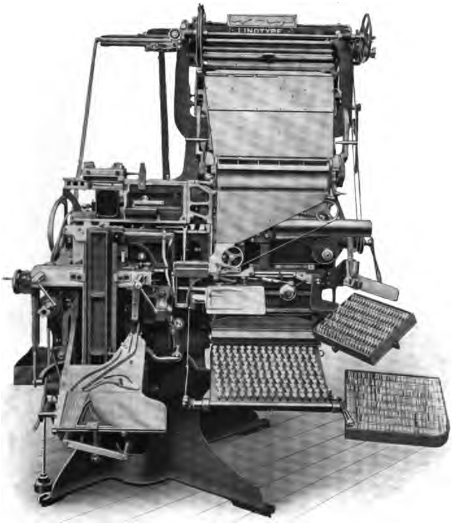
FIG. 407.—Linotype; arabic machine, with 180 keys.
