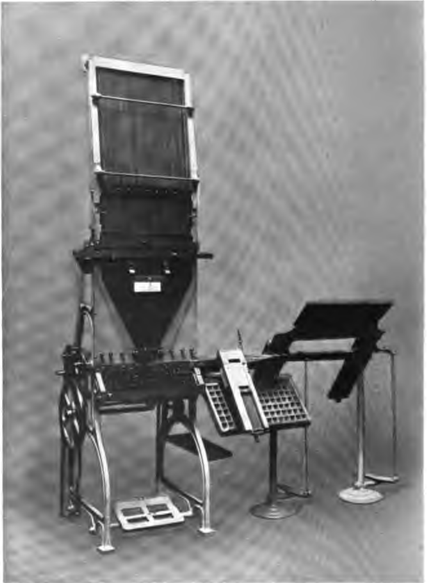
FIG. 311.— Kastenbein composing machine.
