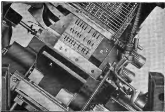
FIG. 443.— Typograph; matrices line-justified ready for casting.
