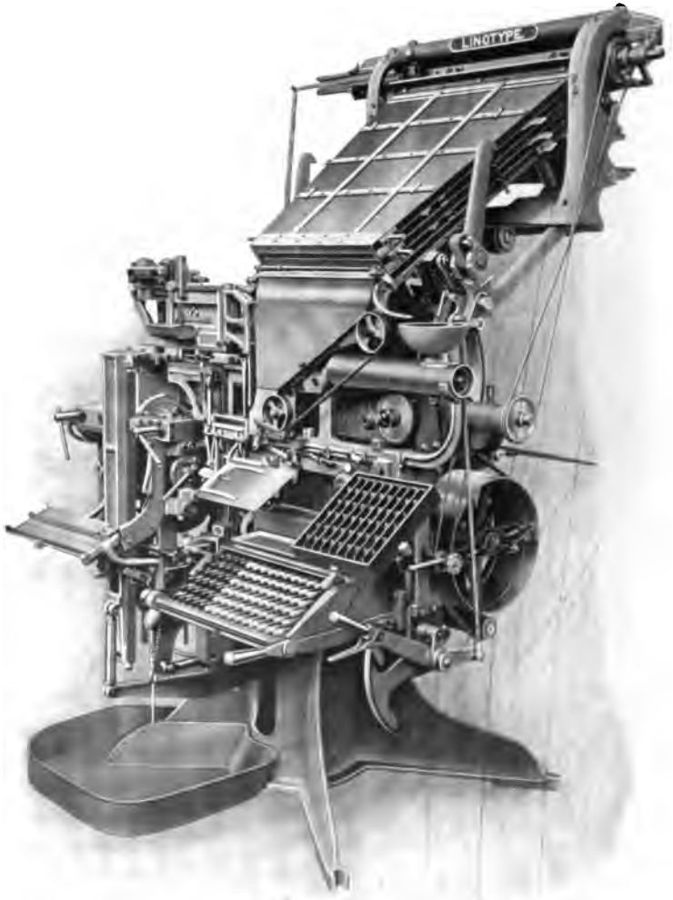
FIG. 408.— Linotype; treble magazine machine; English model 4; front view. To face plate LXIV.]
