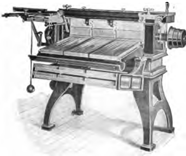
FIG. 333.— Empire automatic distributing machine. [To face page 352.]
