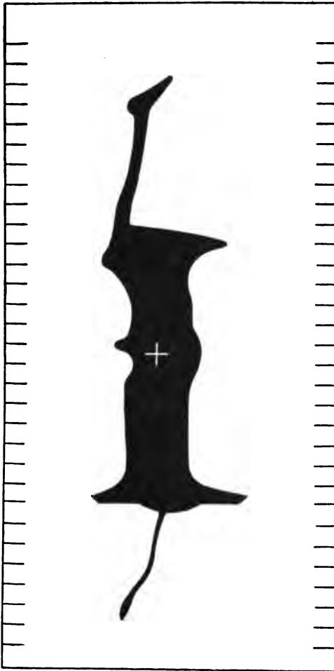
FIG. 142.—Mean resultant character obtained by combining in their proper proportions the whole of the lower-case characters and f-ligatures of an old-style 12-point face. The centre of gravity of the character is marked by the white cross.
