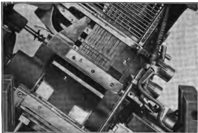
FIG. 442.— Typograph; vice-jaw closed but line not yet line-justified.
