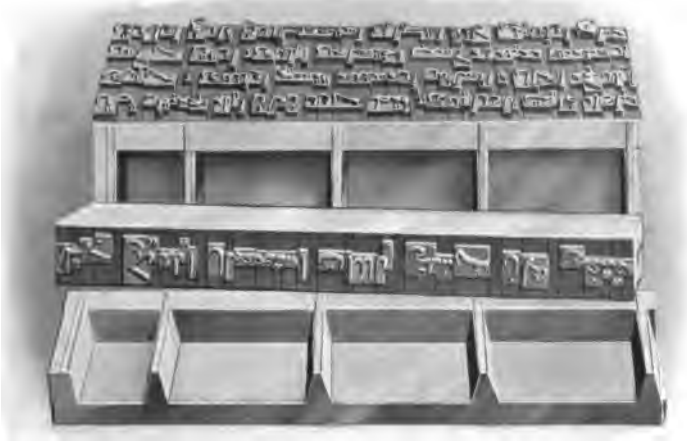
FIG. 243.— Linotype; arabic recessed slugs.
