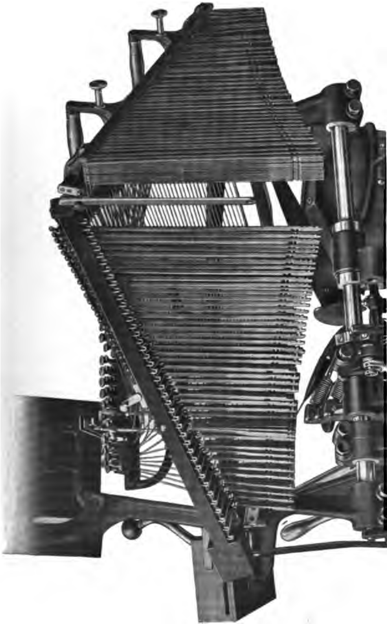
FIG. 445.— Typograph : matrices transferred from magazine to the rack, ready for removal. [To face plate LXXXVIII.]
