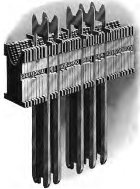
FIG. 415.—Linotype ; composed line of single-letter matrices ready for casting the slug.
