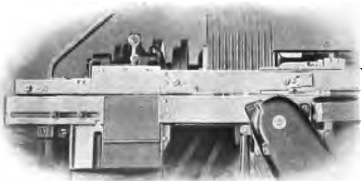
FIG. 347.—Dow composing machine; line of composed type on the bridge; justification in progress. To face page 365.]
