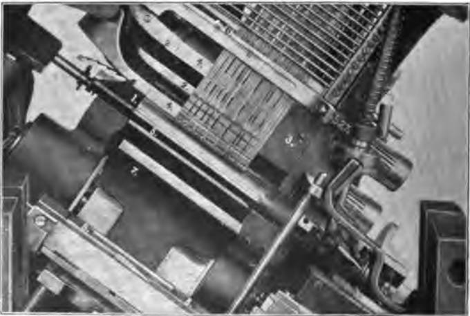
FIG. 441.— Typograph ; assembly channel filled with line of two-letter matrices.
