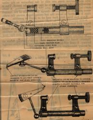
The universal ball joint and the adjustable brackets give this clamp a great range of adaptability as it can be fastened on to any convenient place where accurate testing or indicating is to be done.
