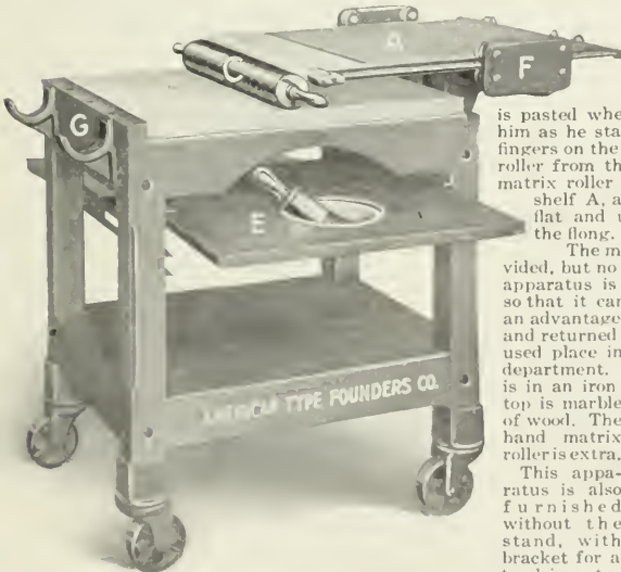
American Matrix Tissue Holder with Matrix Roller in Use
