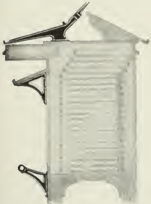
Sectional view of Masterman Composing Room Cabinet showing position of job cases, foot rail, supplementary galley bank, copy-drawer box and the brackets and 18x72 inch bank on top
