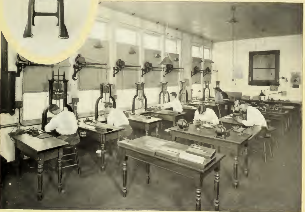
A VIEW OF THE MATRIX CUTTING MACHINES
