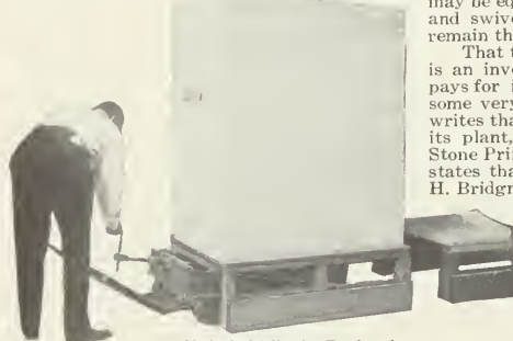
Method of Adjusting Truck under Loaded Platform
