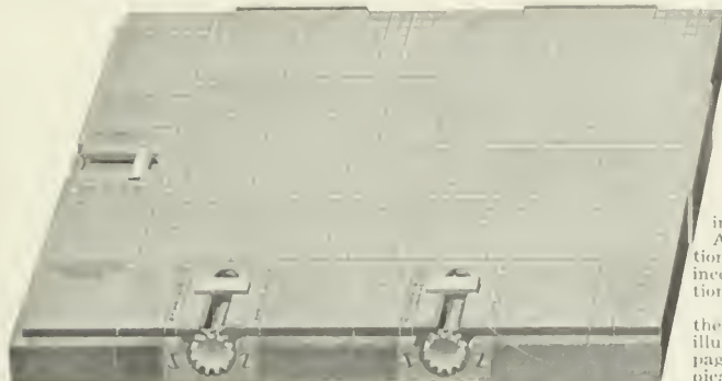
Cut No. 1. Shows page 39x55 picas outside. Three hooks and three brass catches to page. For book or catalogue work.
