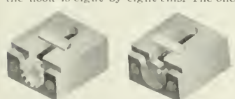
Cut No. 4. Hooks are made of iron and steel. Illustration shows one for hook work with ratchet for quick changing of plates.
