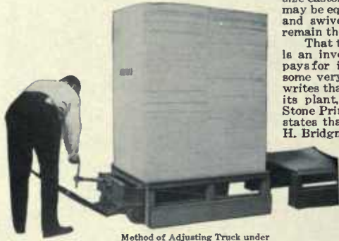
Method of Adjusting Truck under Loaded Platform
