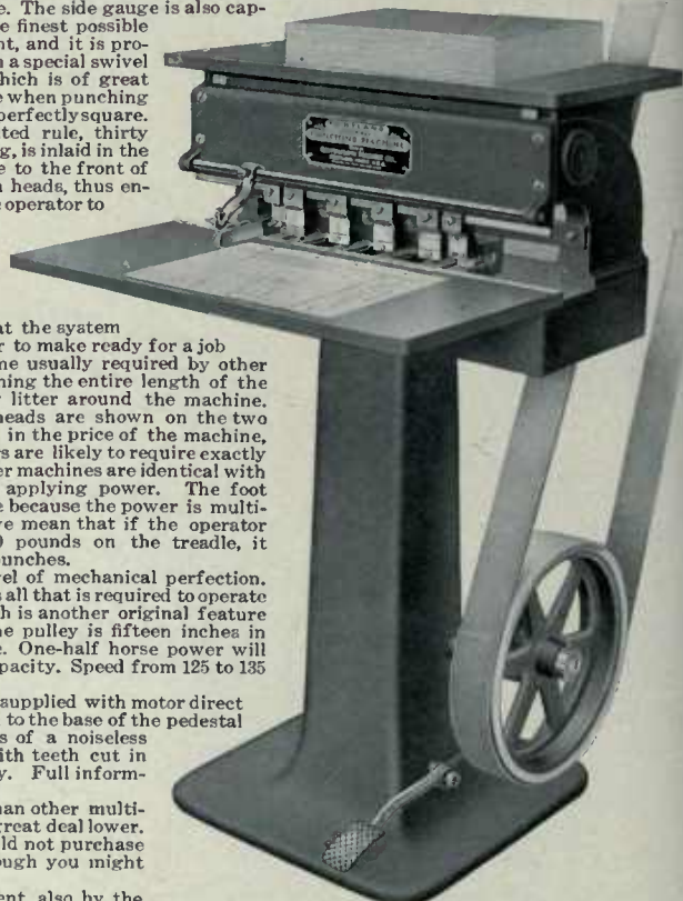
This illustration shows power machine equipped with four open hole Punch Heads Style M1. Punch heads are not included in the price of machine, as no two users are likely to require exactly the same equipment.
