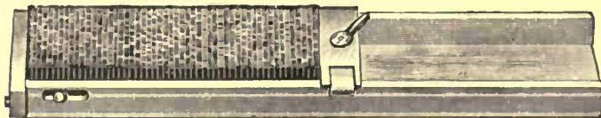
Shows the Galley locked at end and side.
