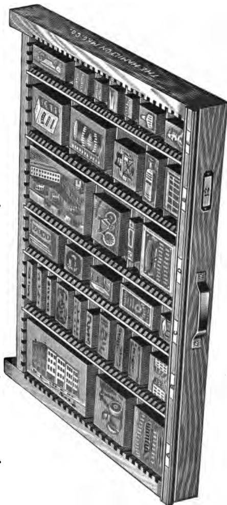
This cut shows a case as it appears when divided off and filled with cuts or electrotypes.
