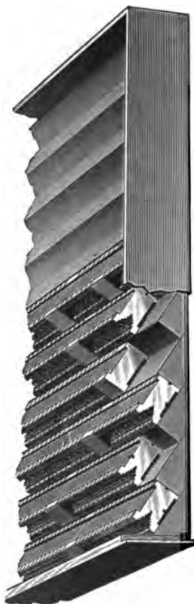
DETAILED SECTION OF MATRIX DRAWER, SHOWING MATRICES IN PLACE.
