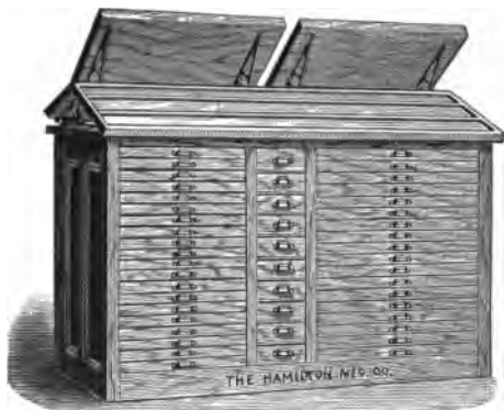
Front View of Polhemus Cabinet, showing Sort Drawers, Galley Top and Job Cases.
