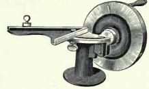
This Mitreing Machine combines simplicity with usefulness, being accurately made and well finished, and mitres brass or metal rule with complete accuracy to any angle.
