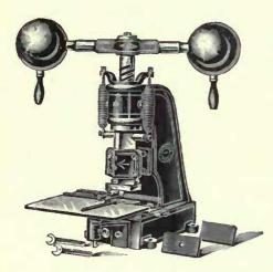
These Presses are of strong construction, and have ample leverage; the method of working them is simple. The Stamp is attached to the Slider Plate, the Case is placed on the Press Table, and on the Press Handle being pulled, the Stamp is forced down upon the case. The Stamp is kept hot by Gas Jets in the Heater Box above it.
