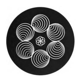
of divisions between each cut. Although the number of divisions through which the division-plate has to be turned can be ascertained by trial, it appears convenient to calculate the number. This may be done in the manner following, in those cases at least in which the outer circles of the shells are in contact.
