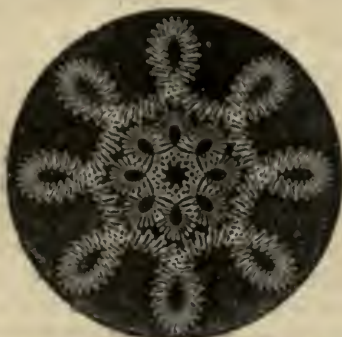
Geometric Chuck combined with the Rose Engine
