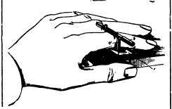
The combination of a base-plate, provided with a standard, a graduated bar provided with a mortise or slot whereby the gradua ed bar may be readily adjusted upon the standard, and a gage stud for adjustment with relation to the standard.
