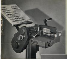
Front view of Supersurfacer. A slug clamped in place for surfacing can be seen in the slug-clamp at the right. Hand-wheel and scale for micrometric adjustment are located within the belt-guard casting at the left. Notice the convenient location of the electric switch and of the slug-tray on the rack.
