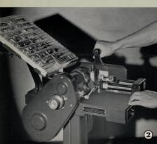
THE LUDY OW SUPERSURFAC designed to take a very light Ludlow sluglines, particularly bolder typefaces. Depth of surf a fraction of a thousandth of justment. Slugs processed by t ror-smooth surface of accurat throughout their entire length, which requires only the minimu
