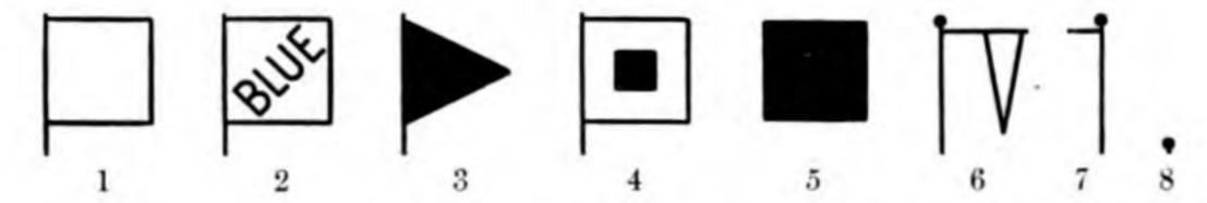
EXPLANATION OF SIGNALS.—No. 1, White Flag, always indicates clear or fair weather, no rain. No. 2, Blue Flag, indicates rain of snow. No. 3, Black Triangular Flag, always refers to temperature; when placed above or before Nos. 1 or 2 it indicates warmer weather; when placed below or after Nos. 1 or 2 it indicates colder weather. No. 4, Cold Wave Flag, indicates the approach of a sudden and decided fall of temperature.
