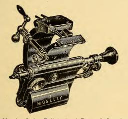
Fig. 116. Moseley Swing Tailstock. 1, Base; 2, Standard Carrying Stops; 4, Swinging Arm Carrying Spindle; 7, 8, Clamp and Set Screw for depth of cut: 9, Spindle; 10, Steady Pin; 13, 14, Nut and Clamp for Feed Screw; removing 14 allows arm to drop forward; 17, 18, Stops or Gauges between which jewel or setting is placed; 18 may be adjusted by rear screws 19; 20, Pivot on which arm swings.
