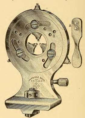
Fig 216. Self centering back rest for the watchmaker's lathe.
