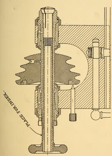
Fig. 24. Longitudinal Section of Head Stock of American Lathe. Full Size.
