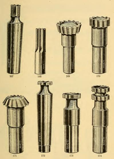
Figs. 167 to 174. Group of end and side cutting mills of shapes suitable for the watchmaker, enlarged to show construction. In cutting sinks, channels, crossing out wheels, etc., the work is held in the face plate, or on a cement brass and swung by hand to feed against the mill when cutting arcs of circles. Straight lines are cut by moving the pivot polisher spindle with the work held by the index pin of the lathe.
