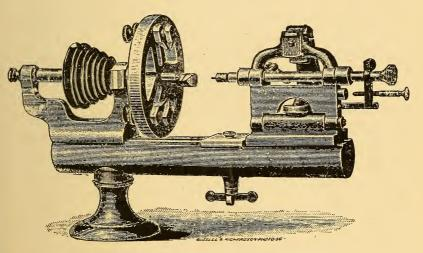
Fig. 15. Earliest Form of Commercial Lathe.
