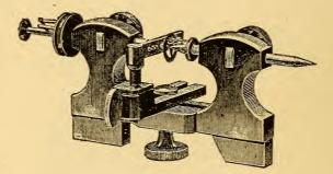
Fig. 10. Dracip Lathe Ready to Drill Pinion.
