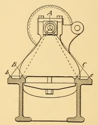
Fig. 17. Sectional View of Engine Lathe.
