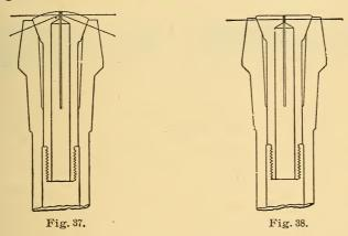
diameters, each section is weak and springs easily. In the flat face the bearing is under the head and the pressure direct as it should be. This is the only correctly designed chuck yet produced. With Dale chucks like this, in full and half sizes, the finest staff and pinion work can be done. We make them for any lathe, from No. 3 to No. 30, and in any size for Moseley No. 2, on account of conoidal design."
