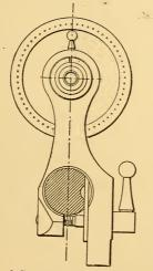
Fig. 23. Section of Geneva Lathe in Front of Headstock. One-Half Size.
