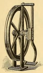
Fig. 223. Oliver Foot Wheel with Double Race and Ball Bearings.
