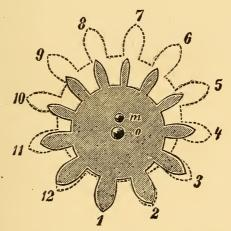
Fig. 213. Shows how a badly centered wheel is left by the rounding-up cutters.
