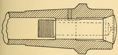
Fig. 25. Enlarged View of Lathe Spindle, showing Chuck Properly Seated. Compare with Fig. 26.
