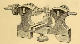
Fig. 9. Dracip Lathe Ready for Drilling.
