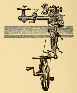
Fig. 219. Modern German Lathe driven by Hand Wheel.
