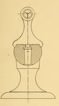
Fig. 22. Section of American Lathe in Front of Headstock. One-Half Size.
