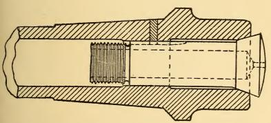
Fig. 26. Enlarged View of Lathe Spindle, showing Chuck Seat too Small. Compare with Fig. 25.
