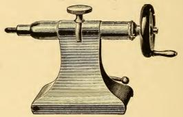
Fig. 112. Screw Tailstock.
