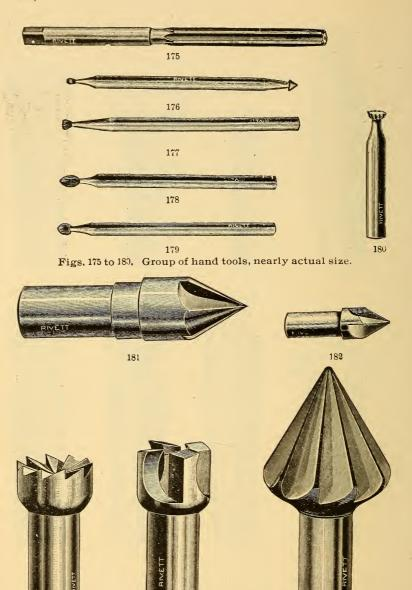
183 184 185 Figs. 181 to 185. Counter-bores and Reamers, enlarged to show construction.
