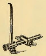
Fig. 197. Latch for Index Plate.
