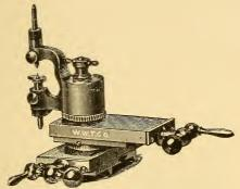
Fig. 211. Rounding-up Tool Bolted on Slide Rest.
