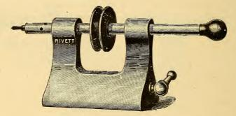
Fig. 114. Traverse Spindle Tailstock.
