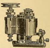
Fig. 195. Moseley 3-Spindle Wheel Cutter to bolt on slide rest; also made with one spindle; the pump center shown at the rear is used to align the cutters with each other and with the lathe center.
