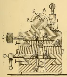
Fig. 103. Cross Section of Rivett Slide Kest. A, Tool Post. B, Elevating Quill. C, Binding Screw of Tool Post Swivel. D, Binding Screw of Swivel between Slides, J, J, Splines, E, Tool.
