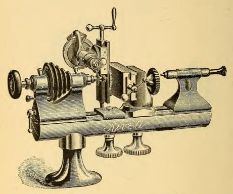
Fig. 201. Rivett lathe arranged for wheel cutting.
