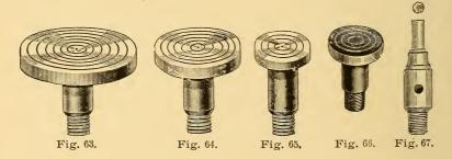
Figs. 63, 64, 65, 66, and 67 show various sizes of these brasses after they have been put in the chuck and turned up true on the lathe by the watchmaker. The rings on the faces of the brasses are added as a guide in placing the wheel before spinning it to center. Fig. 67 shows a  $\frac{1}{4}$ -inch cement brass turned down for small work and a hole drilled in the shank to insert a pin for use as a wrench when
