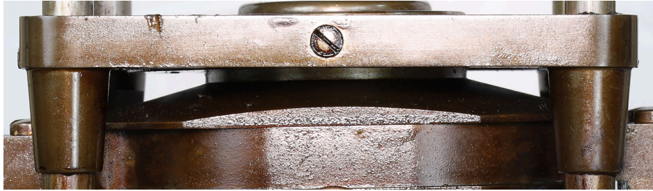
Figure I.4.24: Quill Gimbal Outer Frame, Front View
