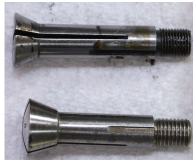
Figure IV.1.32: Moseley No. 1 vs. Lorch 6mm
