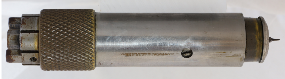
Figure IV.1.30: ATF Quill #53, General View (with cutter)
