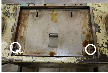
Figure IV.1.5: Base Casting, showing 10.11 Medial motion plate locking studs (circled)
