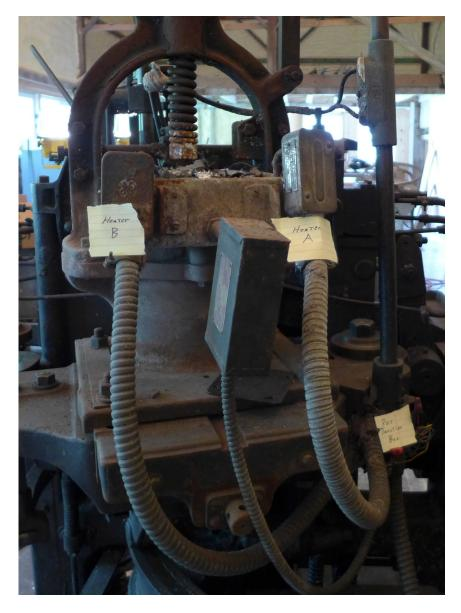
A view from behind the caster of Pot Heater 'A' (on the right in the photo, which is on the left / flywheel side of the machine as viewed from the front) and Pot Heater 'B' (at left in the photo). The Pot Heater Junction Box is labeled at the lower right of the photo. The Pot Heater Lamp Standard goes vertically straight up from this Junction Box.
