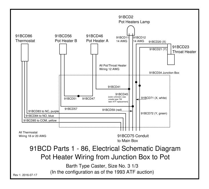
I'll start from the (missing) light on the top of the machine and work down. Here is a photograph showing the Pot Heaters Lamp Standard¹ from the *back* of the caster, together with a highly schematic drawing identifying its parts. This is the Lamp which, when illuminated, indicates that the Pot Heaters are receiving power.
