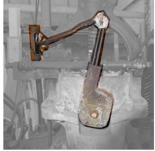
91bCD23 Throat Heater Assembly (right phto) and its wiring from the 91BCD14 Pot Heater Lamp Standard Tee Condulet (left photo) Shown from the front (nipple side) of the Pot, with the Pot swung back.
