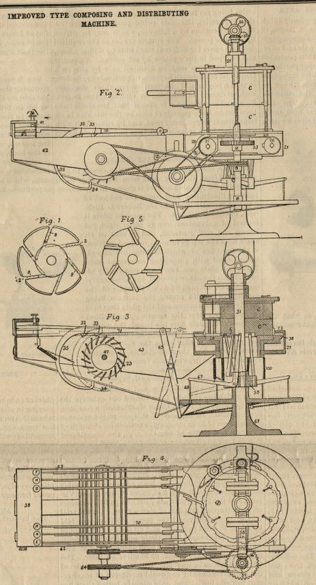
carries a spur wheel, 53, that engages the toothed perimeter of the table, 30. This shaft is driven by means of bevel gears, 56, 57, from a cross shaft, 58, mounted above the machine, and supplied with driving and loose pulleys.
