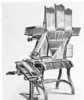
EMPIRE COMPOSING MACHINE, Circa 1880. The first American machine to achieve practical operation. It had somewhat general use until superseded by the Thorne and later by the Linotype. It had a complementary type distributing mechanism.
